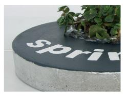
then press slightly with the palm of the hand on the casting object, so that the air penetrates between the casting object and mould. Tap the casting mould gently on your pad, so that the cement-object becomes entirely detached from the mould.
