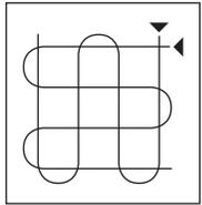
Move evenly and slowly the spray can back and forth, and carry out the turning motion beyond the edges of the object (cross-coat). If necessary, spray a further coat “wet-on-wet” at intervals of 1-2 minutes.
